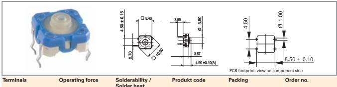
TerminalsOperating forceSolderability / Solder heat resistanceProdukt codePackingOrder no.THT outward3.3±0.6 NE DIN IEC 600 68-2-20A1tubes à 60 piece1.14.100.501/0000
